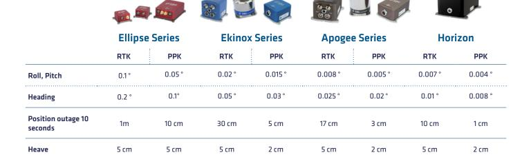
GNSS position accuracy = 1 cm + 1 ppm (RTK/PPK). RTK = Real-time Kinematic. PPK = Post Processing Kinematic. Heading with a 4-meter baseline. RMS values for typical marine survey trajectories, better performance in automotive. Preliminary version. All specifications subject to change without notice.
